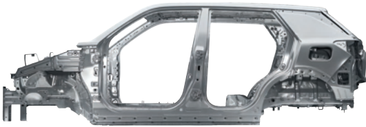
74% صلب 74% High-Tensile Steel
